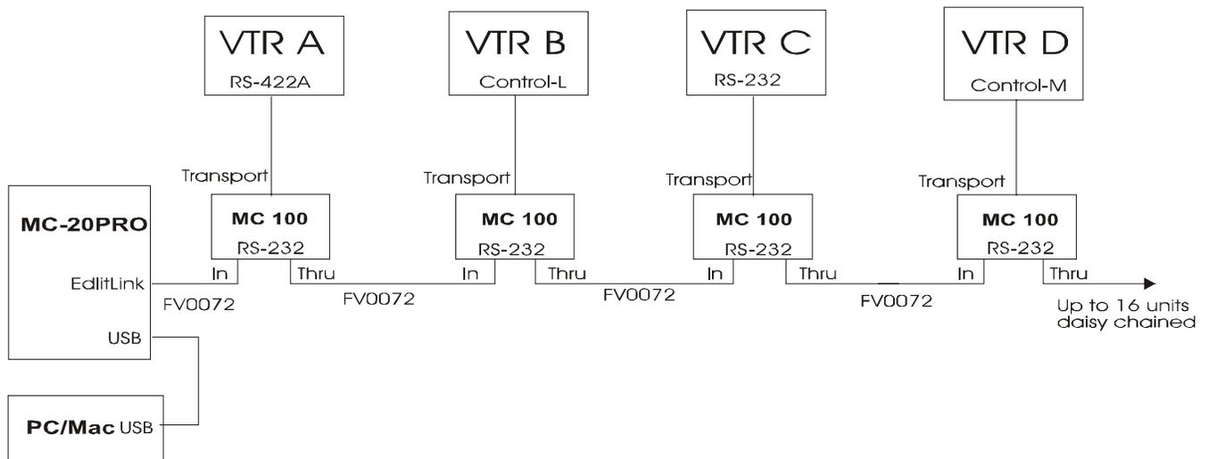
When using the MC-100 controller, ensure the “Slave” mode switch that is behind the panel of the MC-100 is set towards the right. MC-100 units that have a ”Slave” label on the bottom (that were ordered as “slave” units) have this switch pre-set to this position by the factory.
